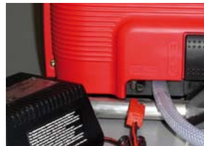
Outside recharging socket
