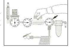
manifold (Item # 78), in the cross line position. The adjustable 100 psi relief valve (Item # 42) will relieve and produce a notable popping sound.
