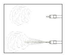
**Helpful Hints:** Occasionally, when working overhead, the pressure exerted on the liquid tank by the regulator will not be sufficient to drive the liquid 8-10 feet above floor level. At this time, you need to increase the pressure on the liquid tank by adjusting the regulator clockwise to the point you receive the aerosol at the tip and at the height you desire to work.
