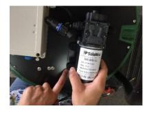
To install pump, you will need to secure the four rubber feet into the main unit first by using the included bolts.
