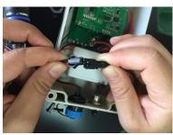
The male and female plug of the battey has to be connected correctly. Check all connections to make sure they are all secure. Screw the cover back on the base and replace the scew hole plugs.
