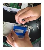
Plug in the battery and secure the battery onto the base to keep it in place by using the two sided mounting tape.
