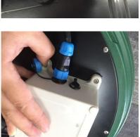
Plug the power cable onto the controller. Screw in the blue connecting nut.
