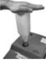
**A**lways use the filler bottle to add water to the machine. The filler bottle is spring loaded to prevent over-filling and will prevent spillage that could damage the electronics.
