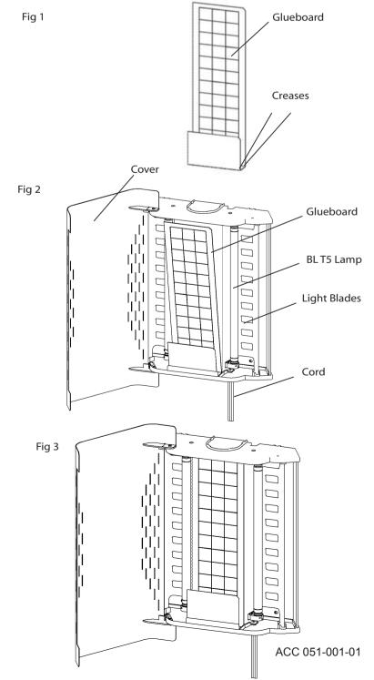
Check the voltage requirements for the flytrap and confirm the correct power source is available. For safe operation it is recommended that the power outlet be fused at 3 amps. This equipment utilises either a standard 110-120v 50/60Hz or 220-240v 50/60Hz outlet with a grounding pin. The power supply must be properly grounded. If in doubt consult a qualified electrician to confirm that that grounding is present.
