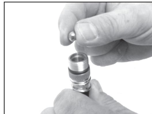
4. Drop new Brass Ball into Inlet Bushing.
