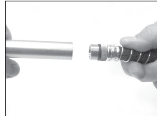
1. Remove Pump Inlet Bushing from Pump Cylinder.
