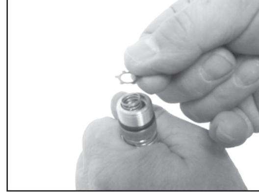
6. Place the Stainless Steel retaining Ring over the opening in the Bushing. Note that the Ring is not perfectly flat.
