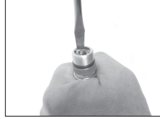
7. Push the Retaining Ring into the Bushing and against the Retainer Seat. Retaining Ring may be seated by using the Shank of a 1/4" Drill or any blunt tool which will not bend or otherwise damage the Retaining Ring.
