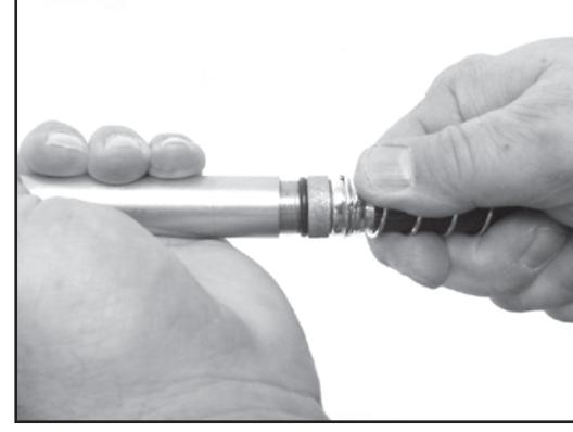
8. Reassemble Inlet Bushing to Pump Cylinder.
