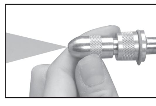
Adjust spray pattern by turning nozzle cap. Do not turn cap more than 2 turns or cap may come off allowing spray material to spray back on you.
