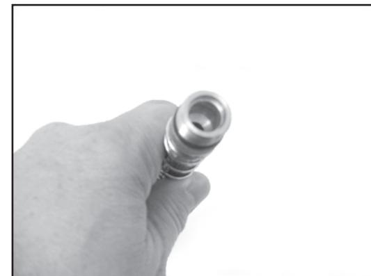
3. Clean interior of Inlet Bushing to remove scale, corrosion products, spray material, etc.
