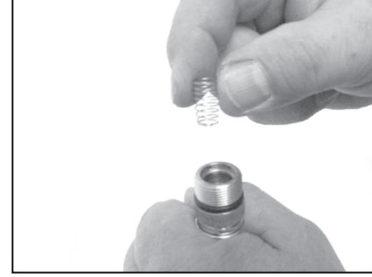
5. Place the Tapered spring in the Bushing with the small end against the Ball.
