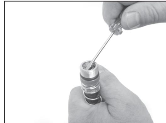
2. Remove old Tapered Spring and Brass Ball.
