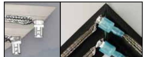
Use the very tip of the ratchet Crimp Tool to crimp the Flag Connector. This will insure a tight connection to the braid. This connection can be tricky so we suggest that you "Tug" on the end to insure that the Flag connector is secure.
