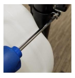
Secure the Wire Clamps on the Handle and Lower Frame using the Phillips Screwdriver.
