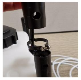
Align the Handle and Wire Clamp with the Lower Frame. Slide the Wire Clamp over the Lower Frame, and the Handle into the Lower Frame.
