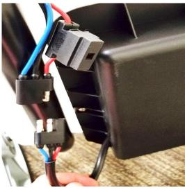
Locate the Wiring Harness Connector at the base of the Handle. Locate the Connector exiting the Back Panel, and connect it to the Wiring Harness Connector, making sure it is fully seated.
