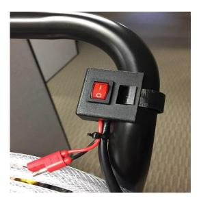
Locate the Switch on the Upper Handle and make sure it is in the OFF (O) position as shown.
