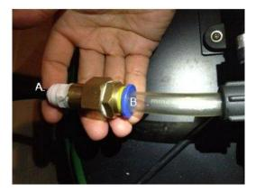
DO NOT ATTEMPT TO REMOVE TUBE FROM POINT "A". **Once you have inserted the tubing in "A", it cannot be removed.** However, you may remove the tubing from point B. (Above)
