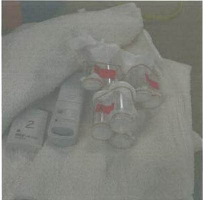
Figure 3. Picture of the insulated environment, including three replicates of each bed bug life stage, a HOBO® data logger, and the indoor/outdoor thermometer.
