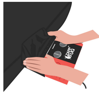
Stretch Tube Around Heating Unit (Observe "Do Not Cover" markings)
